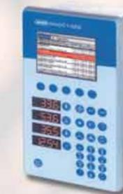
The processor controller IMAGO has a 5" color display. Texts, process values, background diagrams and icons can be arranged as required.
